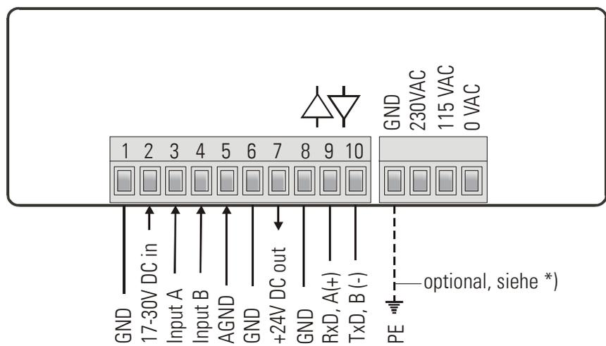
\*) The connection of PE is optional and not necessary for safety or for EMC.
