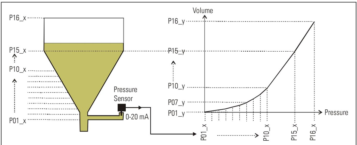
To solve the problem, we divide the non-linear part of the tank into 14 parts. We enter the expected display values of the pressure sensor to registers P01\_x to P15\_x. For the linear part of the tank it is sufficient to store the final pressure value to register P16\_x. Now we can easily calculate the appropriate filling quantities and enter these values to the registers P01\_y to P16\_y.
