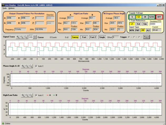
In the Fast Mode the Oscilloscope wave form is auto scaling, as a result the 4 wave forms remain the same over the full frequency range.
