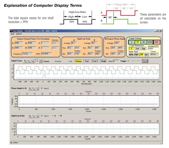
In the Fast Mode the Oscilloscope wave form is auto scaling, as a result the 4 wave forms remain the same over the full frequency range.
