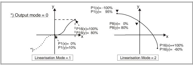
You can visualize your curve on the PC screen or by means of an external oscilloscope. For this, select TOOLS, then TEST and there "Analogue Voltage Function". The unit will now simulate a repeating frequency course over the full range and generate the analogue signal accordingly. When you use the Scope function of the operator software, you must set the serial code to "<u>:1</u>" to record the analogue output.
