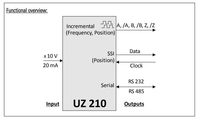
The unit accepts analogue input signals (0 -  $\pm$ 10 V, 0 - 20 mA or 4 - 20 mA) for conversion to digital output signals.
